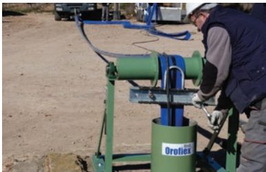
A single Oroflex Well hose can accommodate depths up to 990 ft.
