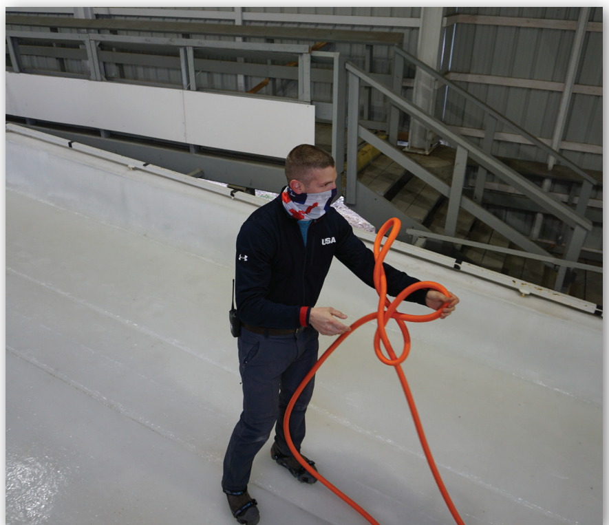
John Napier testing the Tundra hoses' kink resistance.
